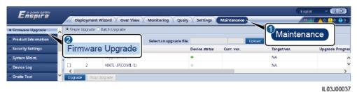
Tab **Function Operation Description** 1. Select the upgrade package Single Upgrade Upgrade a device of any type. and click **Upload**. NOTE 2. Select the device that requires The Single Upgrade mode does not a firmware upgrade. apply to two or more types of device at a time. For example, you 3. Click Upgrade. cannot select both SUN2000 and MBUS. 1. Select the upgrade package Batch Upgrade Upgrade solar inverters in and click Upload. batches. 2. Click Upgrade.
