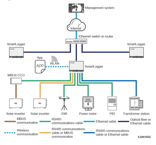
Figure 2-4 Fiber or Ethernet star network
