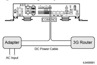
**Step 2** Choose **Settings** > **Other parameters** and set **Reset the external router** to the DO port.
