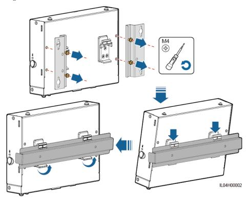
Figure 3-3 Guide rail-mounted installation
