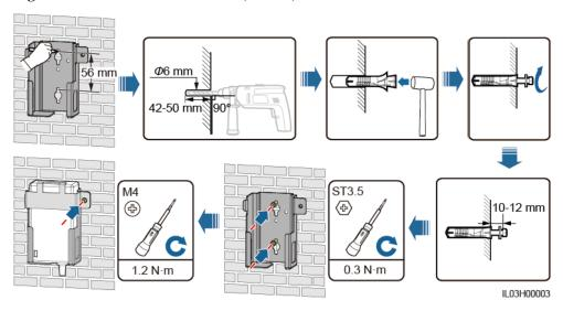
Figure 3-10 Wall-mounted Installation (Mode 2)
