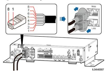
Figure 4-10 Connecting an Ethernet cable
