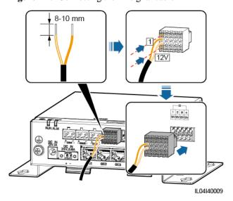
Figure 4-19 Connecting the DI signal cable
