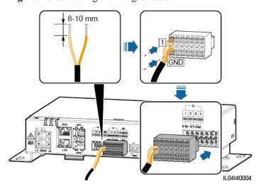
Figure 4-8 Connecting the AI signal cable
